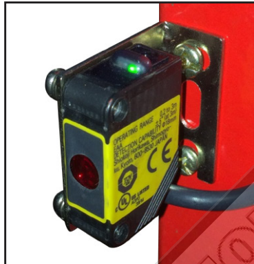
Power on & not aligned
